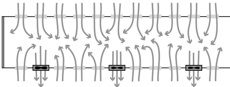
**Figure 4. Minimum ventilation setup uses various combinations of 36-inch and 48-inch fans, depending on ventilation rate needed. Object is to bring air in through vent boxes to mix with warm inside air, and avoid chilling birds. Note: Light traps and false wall not shown here.**
