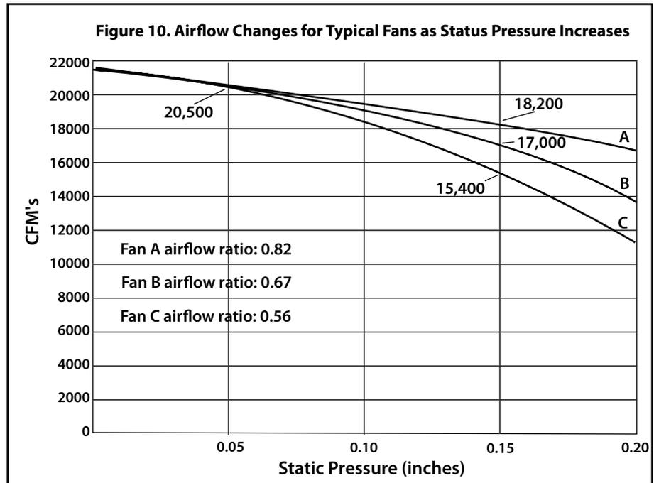
The greater the light trap area, the lower will be the static pressure drop across the trap and the load on the fan. A false wall tunnel fan room allows using larger light trap area, for lower static pressure.
