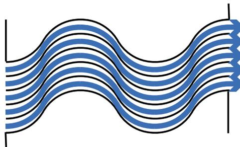
**Figure 8. One type of commercial light trap is called variously an “S,” “W,” “blade” or “vane” trap. This type trap, if well designed, can block light well without overly restricting airflow.**
