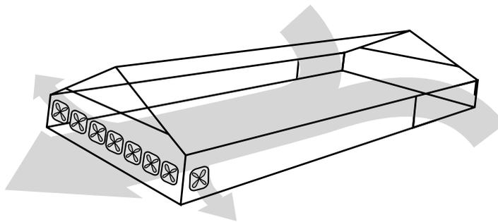
**In hot weather tunnel ventilation can reduce the “effective” temperature by 10-12 degrees F, but must be used with care when birds are young.**
