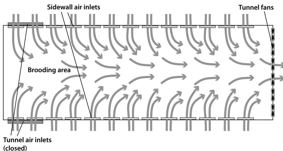
Figure 6. Transitional ventilation uses the same basic setup as in minimum ventilation. The difference is that ventilation is thermostat controlled in transitional mode, not timer controlled. Note: Light traps and false wall in tunnel fan end not shown in this diagram.
