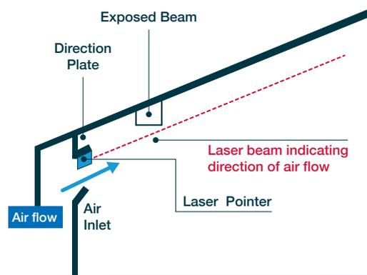
Direction plate in correct position. Laser pointer shows air flow will bypass exposed beam and continue to rood apex.
