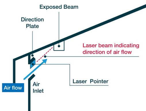
Laser pointer indicates direction plate not in correct position. Air will be deflected by the beam and fall onto birds.
