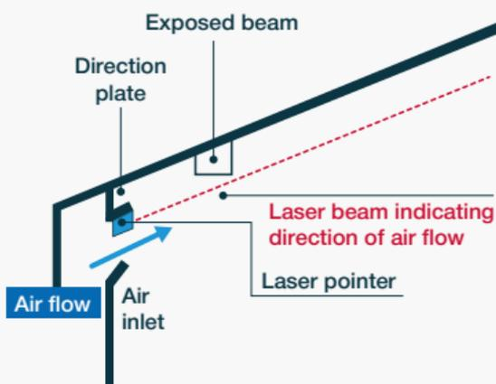
Direction plate in correct position. Laser pointer shows air flow will bypass exposed beam and continue to the ceiling apex.
