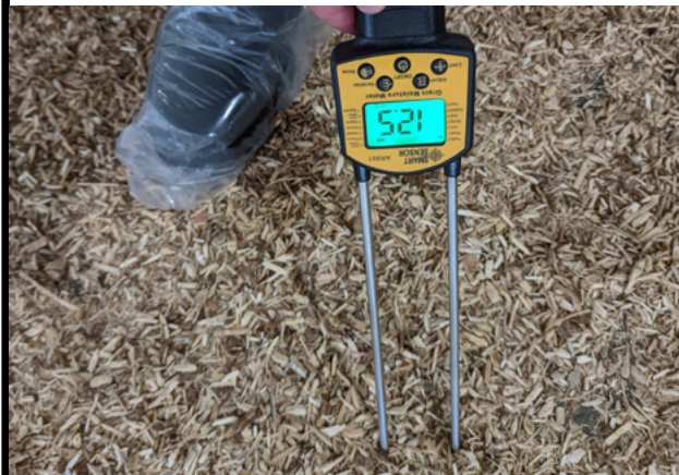
Figure 6.32 Litter moisture measurement.
