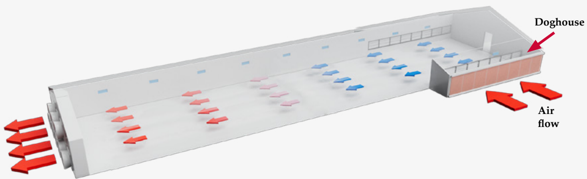
Figure 6.18 Air flow in a tunnel-ventilated house.
