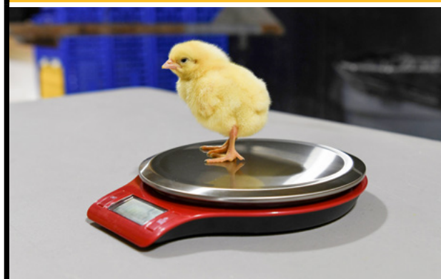
Figure 3.8 Electronic platform scales for individual bird weights up to 7 days of age.
