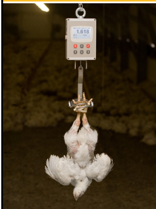
Figure 3.3 Individual bird weighing with an electronic scale.
