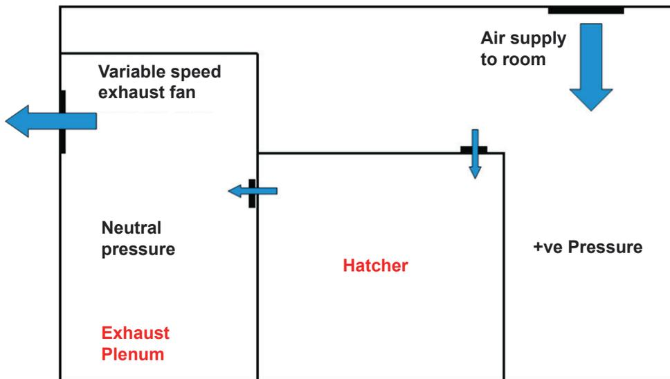
In the above situation, the hatcher exhausts through the rear of the machine directly into the exhaust plenum.
