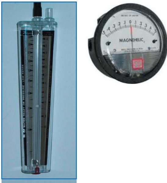
All pressure meters should have 2 ports/terminals - one for positive pressure and one for negative pressure.
