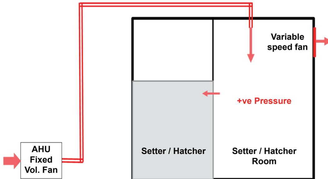
It is important for the capacity of the variable speed fan to be correctly determined during design. A typical fan configuration used for this application is shown below. The fan should have shutters on the outside and a weather hood/cowl.
