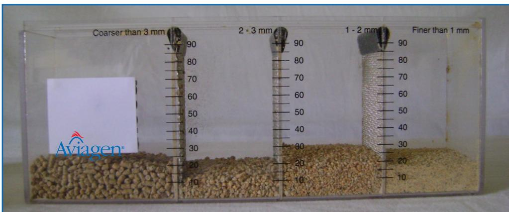
**Figure 4:** Sieving feed on farm before it enters the hopper to reduce percentage of fines presented to the birds.
