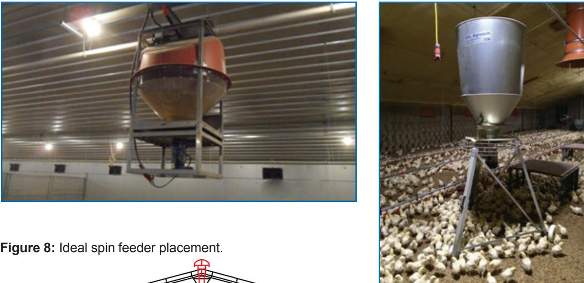
**Figure 8:** Ideal spin feeder placement.
