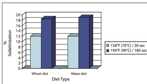
Figure 5 clearly shows that increased conditioning time and temperature increases gelatinization in feed, regardless of the cereal base used. The process of gelatinization creates natural 'glues' which allow the feed particles to compress tightly and adhere to each other when passing through the pellet die. Optimal 'cooking' of feed will result in more durable pellets and reduce levels of fines (Figure 6).
