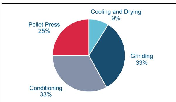
Grinding of raw materials and conditioning of feed are regarded as the most influential factors affecting pellet durability (Figure 4).
