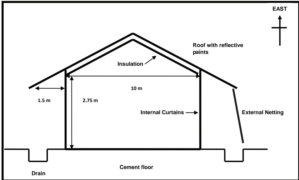
**Figure 17:** Example of a typical open-sided house for broilers grown on slats.
