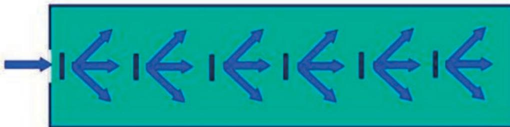
Fans may also be placed to blow diagonally across a house from the prevailing wind side (around 60 degrees from the sidewall – **Figure 30**). In this case, curtains should be fully open on both sides of the house when the fans are operating. Fans should not be placed too close to any objects or sidewalls as this may reduce efficiency.
