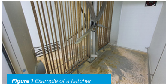
Figure 1 Example of a hatcher cooling coil covered with chick fluff.
