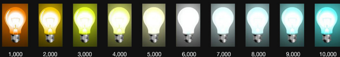
Figure 6.28 The Kelvin scale for measuring color temperature.
