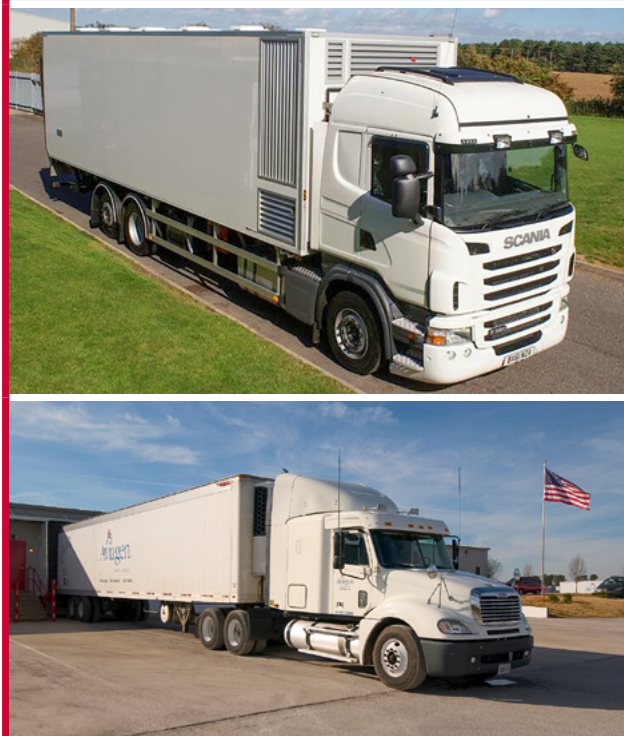
Figure 2.1 Typical controlled-environment chick delivery vehicles.
