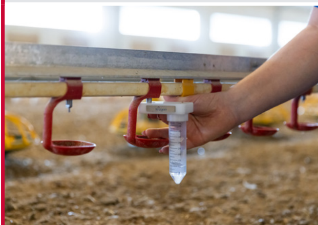
Figure 5.6 Measuring nipple line flow rates.
