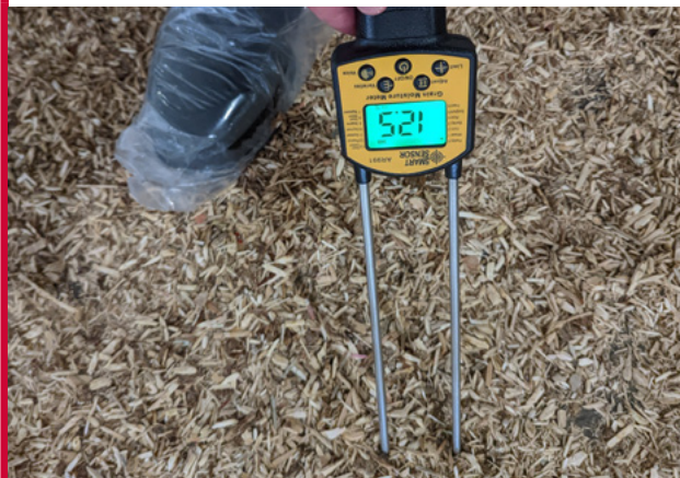
Figure 6.32 Litter moisture measurement.
