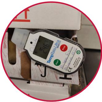
The temperature at DOC box level can be checked by reading the temperature data logger attached to an outside box with pink tape.
