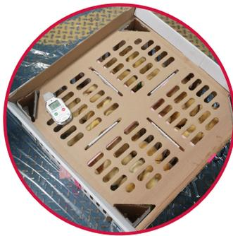
The temperature inside the DOC box can be measured using any reliable temperature meter.
